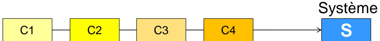
$$R_s(t) = R_{C_1}(t) \times R_{C_2}(t) \times R_{C_3}(t) \times R_{C_4}(t)$$
